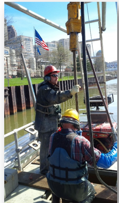
Sediment sampling within the Cuyahoga River federal navigation channel, September 2015
